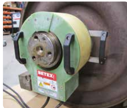
Heating bearing rings for dismantling
