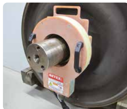
Heating labyrinth rings for dismantling
