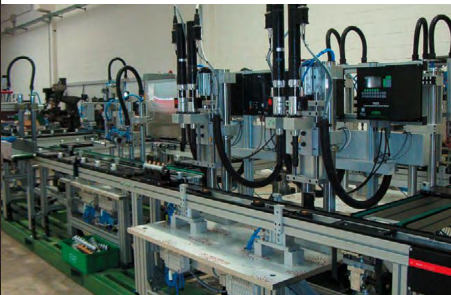
Pallets automatic line to fasten the screws on thermo-hydraulic collectors
