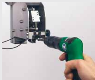
The photo shows the automatic screw picking with a Fiam air tool
