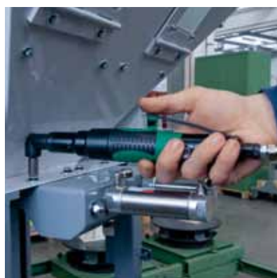
Reaction on the hand (torque reaction)
