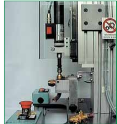
Workstation for the tightening/un-tightening of industrial valves
