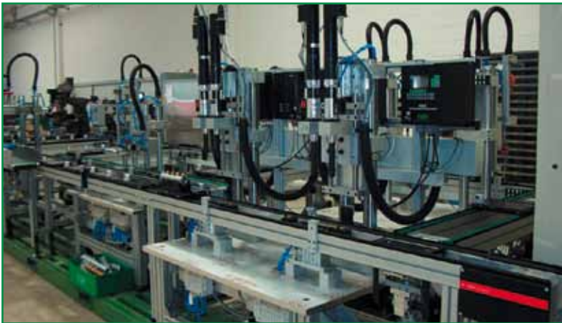
Pallets automatic line to fasten the screws on thermo-hydraulic collectors
